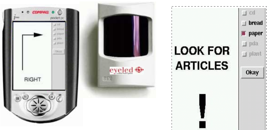
Fig. 2. The hardware of the PDA-based shopping guide (Left: Example display on the PDA, which receives location signals from a beacon (middle). Right: Close-up of part of the display in the situation where the user has arrived at a relevant store. \mathcal{U} checks off the items found in the current store and clicks “Okay” to proceed with the next navigation recommendation)
