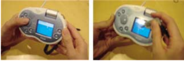
Fig. 1. A small sized display device which enables users to interact with a key and with a pen
